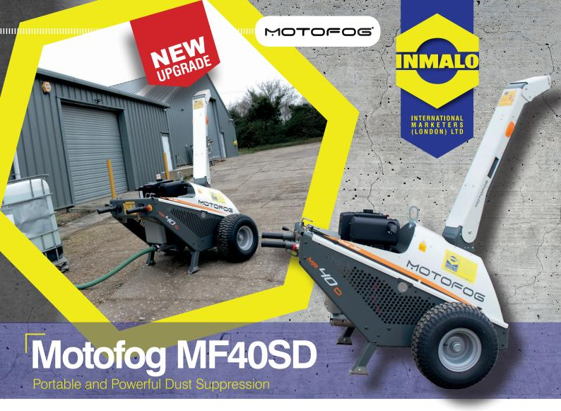
The latest Motofog MF40SD dust suppression unit is a compact, portable and powerful unit for larger demolition sites. It comes fitted with a tried and tested Yanmar engine and only needs connection to a water supply to throw water 35 metres!
